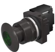
30mm BlackMax, Epoxy Coated Corrosion Resistant Complete Metal Unit Illuminated Push-Pull Operator Full Voltage, 6V AC/DC Incandescent Lamp Mushroom Head Cap Small 1 3/4" (44.5 mm) Metal, Black with Green Lens 3 Position Pull-Momentary/Push-Maintained UL Listed, CSA Certified NEMA 1,3,3R,4,4X,12,13 & Automotive Standards
