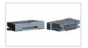
Connector System: Flex-to-Board Number of Positions: 13 Centerline (Pitch): .5 mm [ .02 in ] Insertion Force Type: Zero Insertion Force (ZIF) PCB Mount Orientation: Right Angle
