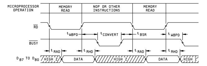
NOTE: For device types 01 and 02, t<sub>RAD</sub> timing is measured at +2 V and +0.8 V.
