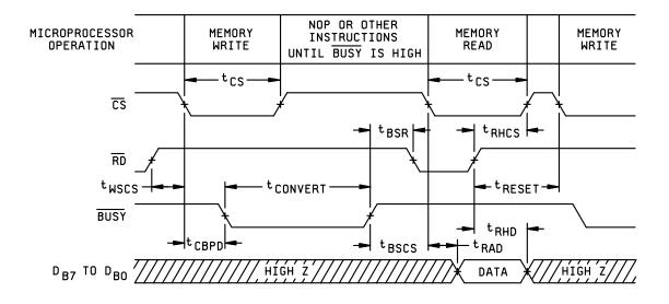
FIGURE 3. Timing waveforms.
