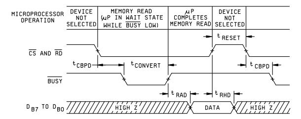
Note: For device types 01 and 02,  $t_{RAD}$  timing is measured at +2 V and +0.8 V.
