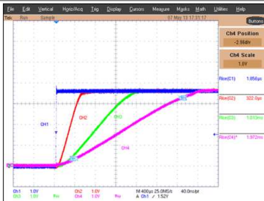
Figure 25. +Power up with different slew rate settings
