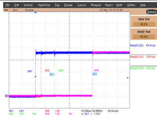
Figure 26. Power up with different tD settings
