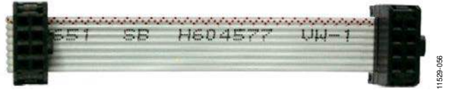
Figure 55. Parallel Cable to Connect Two Evaluation Boards
