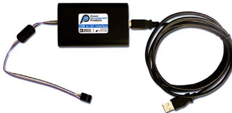
Figure 5. ADP-I2C-USB-Z USB-to-I 2 C Interface Connector
