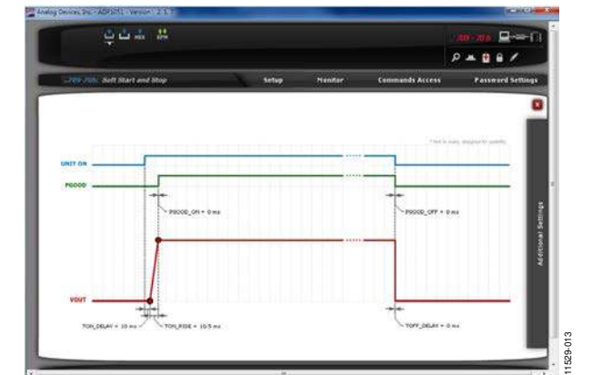
Figure 13. Soft Start and Stop Settings Window
