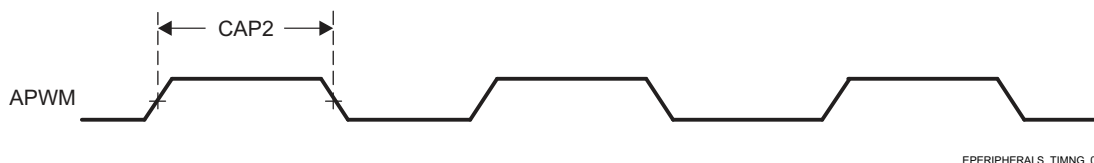
Figure 7-30. ECAP Switching Characteristics
