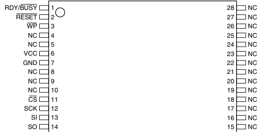
Figure 2-1. TSOP Top View, Type 1
