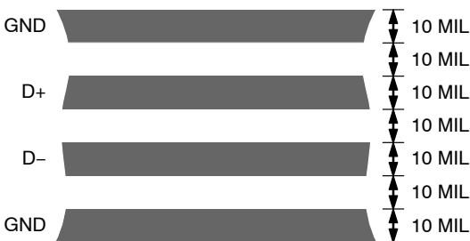
Figure 18. Typical Arrangement of Signal Tracks
