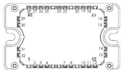
All multiple inputs and outputs must be shorted together Example: 13/14; 29/30; 22/23 ...
