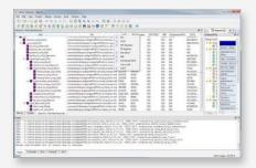
In addition to showing the design hierarchy, important information is available here such as source files used, and both post-synthesis and post-map resources used.
