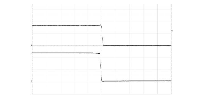
Output disabled by removing V_i at: T_{P1} = +25^\circ\text{C} , V_i = 24\text{ V} , I_o = 4.5\text{ A} electronic load. Top trace: output voltage (2 V/div.). Bottom trace: input voltage (10 V/div.). Time scale: (1 ms/div.).
