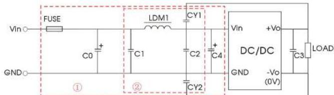
Notes: Part ① is used for EMC test and part ② for EMI filtering; selected based on needs.
