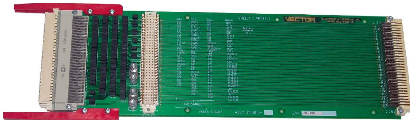
3U, VME64x J1 with 5-row, 160 positions DIN 41612 style connectors (click on image to enlarge)
