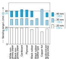
These bars indicate the sensing range with the respective objects when the distance adjuster is set to a sensing range of 40 mm 1.575 in, 30 mm 1.181 in and 20 mm 0.787 in long, respectively, with white non-glossy paper.
