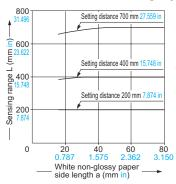
These curves show the characteristics with the maximum sensing range set to 700 mm 27.559 in, 400 mm 15.748 in and 200 mm 7.874 in, with white non-glossy paper (75 × 75 mm 2.953 × 2.953 in).
