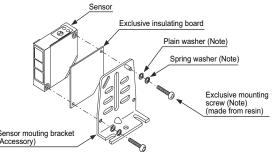
Note: Attached with the exclusive insulating board.
