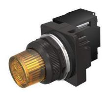
30mm BlackMax, Epoxy Coated Corrosion Resistant Complete Metal Unit Illuminated Indicator Light Full Voltage type, 6V AC/DC Incandescent Lamp, BA9s Glass Lens, Amber UL Listed, CSA Certified NEMA 1,3,3R,4,4X,12,13 & Automotive Standards
