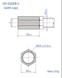
Note: When attaching, make sure that the side without a bearing chamfer is the impact surface.
