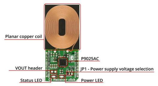
Qi Receiver click relies on the wireless power transfer standard, developed by the Wireless Power Consortium, to both provide and monitor current and voltage. This standard involves digital communication, used to transmit the information back to the charging pad. Depending on the received information packets, charging pad regulates the strength of the variable magnetic field, which in return generates more or less power on the receiver coil.
