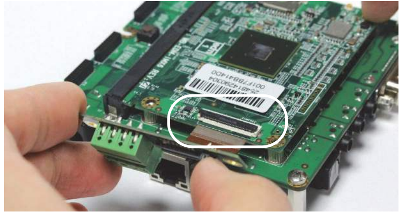
Figure 31: Connecting adapter board and embedded board
