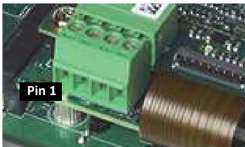
Figure 7: Adapter for Wandboard i.MX6 | I/O terminal, wiring diagram
