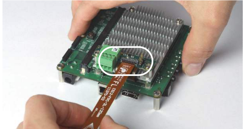
Figure 38: Connecting the camera FPC cable
