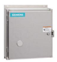
Mechanically held lighting contactor, Contactor amp rating 30Amp 0NC  $\_$  3NO poles, 277VAC 60HZ coil, Non-combination type, Encl NEMA type 4X 304 S-steel Water/dust tight noncorrosive
