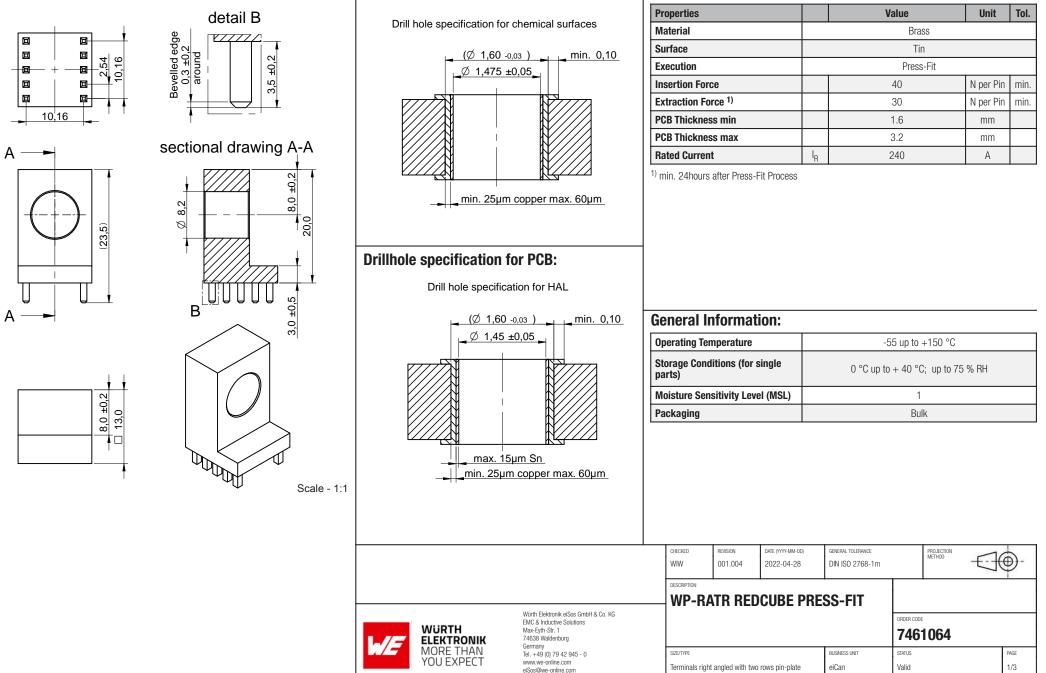
**Drillhole specification for PCB:**
