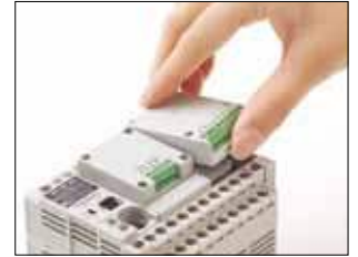
Easily removable (two screws secure the unit)
