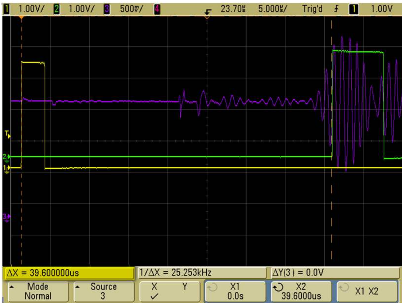
Figure 5-7. START and STOP Signals on Oscilloscope
