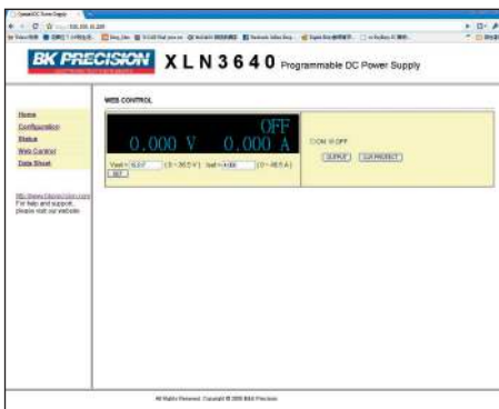
Interface for controlling voltage, current, and output state.
