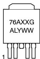
NCV4276A DPAK 5-PIN DT SUFFIX CASE 175AA
