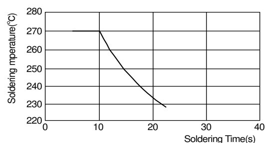
[Allowable Flow Soldering Temperature and Time]
