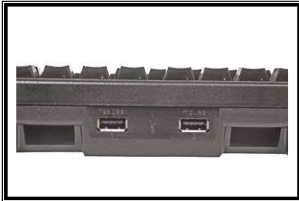
Down Stream ports
