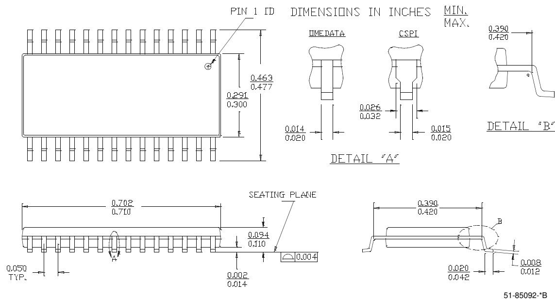
**28-lead TSOP 1 (8 x 13.4 mm) (51-85071)**
