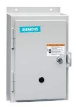
Reversing NEMA contactor Size 1 Three phase full voltage Contactor amp rating 27Amp 3 w 220-240/440-480VAC 60HZ coil Non-combination type Enclosure NEMA type 12 Dust/drip proof for indoors Standard width enclosure
