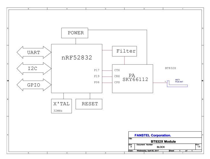
A firmware configuration example to control Skyworks SKY66112 power amplifier is below. This firmware file, SKY66112\_PAconfig.txt can be downloaded from <a href="http://www.fanstel.com/download-document/">http://www.fanstel.com/download-document/</a>.
