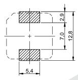
no sensitive traces underneath the component
