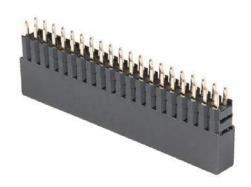
**Description:** This 2x20 "tall" header has the same number and spacing of pins as a Raspberry Pi and provides your board with the ability to extend the heights of your GPIO to accommodate for enclosures or other parts that can encapsulate your Pi. This through-hole header has 40 0.1"-spaced pins and can just be snapped into place with minimal soldering to an applicable "shield."
