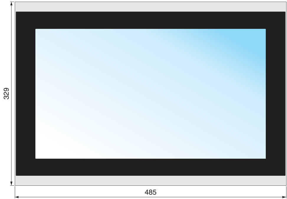
Figure 2-7 Front panel (dimensions in mm)
