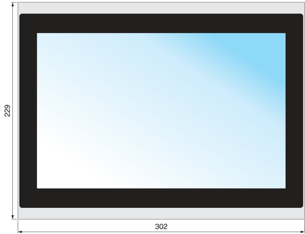
Figure 2-5 Front panel (dimensions in mm)
