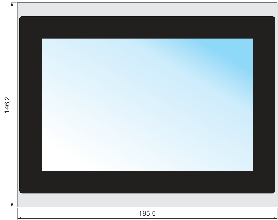
Figure 2-3 Front panel (dimensions in mm)
