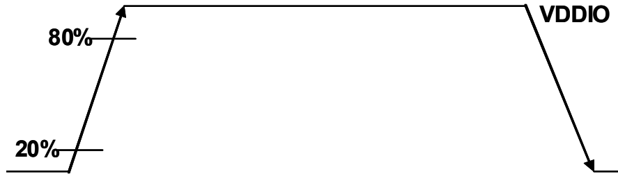
Figure 4. Output Pad Transition Waveform
