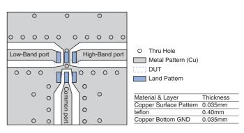
Line width should be designed to match  $50\Omega$  characteristic impedance depending on PCB material and thickness.
