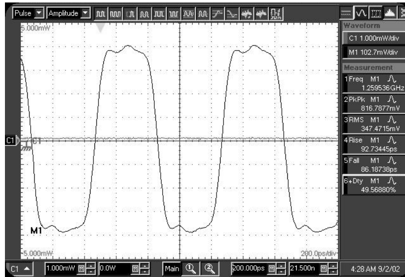
Figure 14 - Differential output with small input amplitude waveform VCC = 4.75 V, Vin = 10 dBm, Fin = 5 GHz
