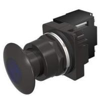
30mm BlackMax, Epoxy Coated Corrosion Resistant Complete Metal Unit Illuminated Push-Pull Operator Full Voltage, 24V AC/DC LED Lamp Mushroom Head Cap Small 1 3/4" (44.5 mm) Metal, Black with Blue Lens 3 Position Pull-Momentary/Push-Maintained UL Listed, CSA Certified NEMA 1,3,3R,4,4X,12,13 & Automotive Standards
