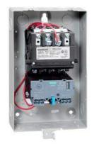
Non-reversing motor starter, Size 0, Three phase full voltage, Solid-state overload relay, OLR amp range 0.25-1A, 208VAC 60Hz coil, Non-combination type, Enclosure type 12, Dust/drip proof for indoors, Standard width enclosure
