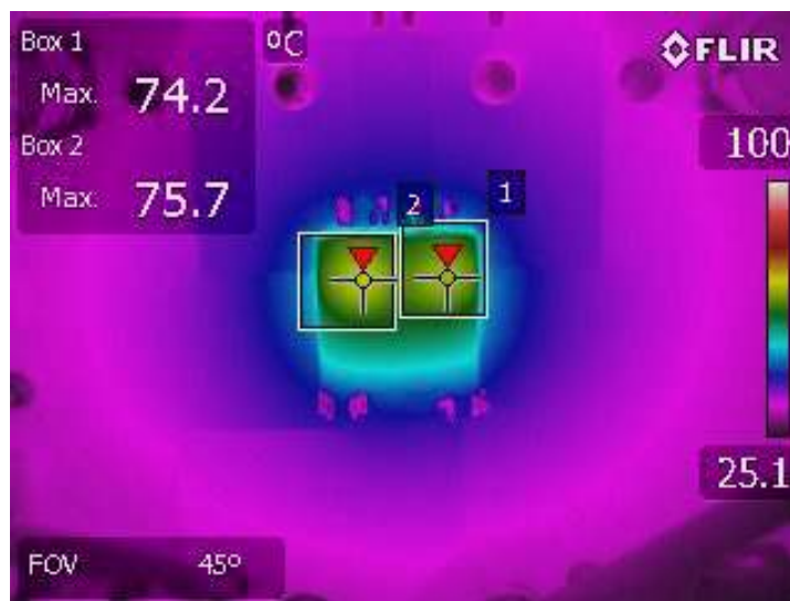
Figure 10. Thermal Image 12V to 1.0V, 36A with 200LFM without Heat Sink
