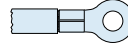
Lug Terminal for Attaching Receptacle Covers to a Panel with a Screw
