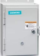
Non-reversing motor starter, Size 0, Three phase full voltage, Solid-state overload relay, OLRelay amp range 5.5-22a, 24VAC 50-60HZ coil, Non-combination type, Enclosure type 12, Dust/drip proof for indoors, Extra-wide enclosure
