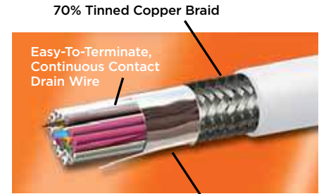
Triple-Laminate Foil with 25% Overlap
