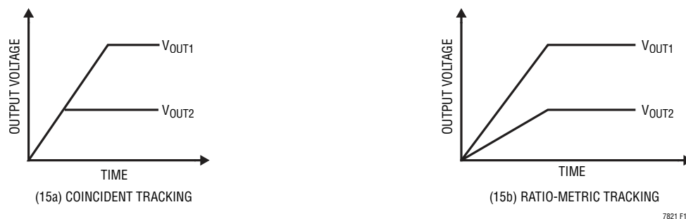
Figure 15. Two Different Methods of Output Voltage Tracking
