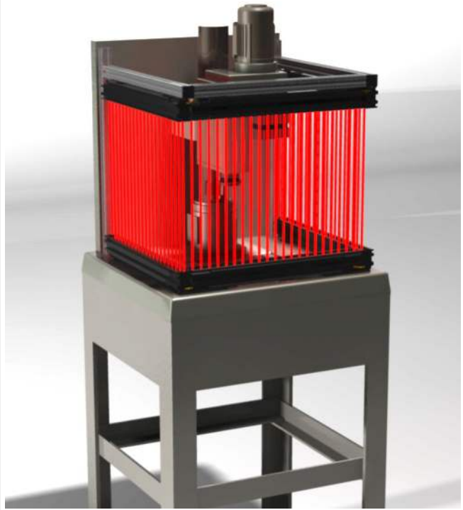
Figure 50. Cascaded light screens guarding a u-shaped cell
