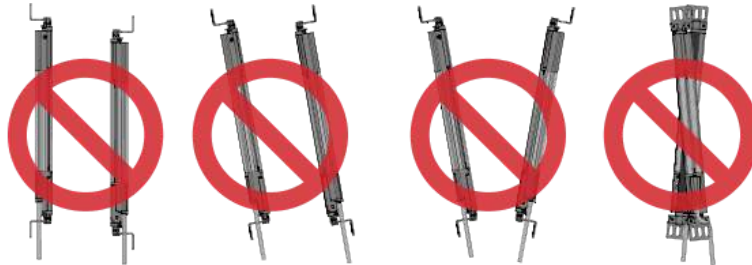
Figure 26. Incorrect Sensor Alignment
