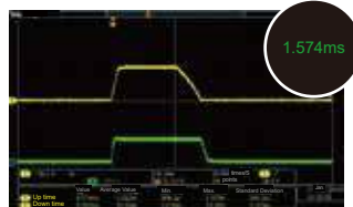
8 sets of IT6522C paralleling together Voltage ratings: 80V Current ratings: 960A Load current: 300A
