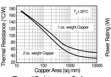
$T_A = 25^{\circ}C$ 2 oz. weight Copper 1 oz. weight Copper 0L 10 100 1000 10000 Copper Area (sq mm)
