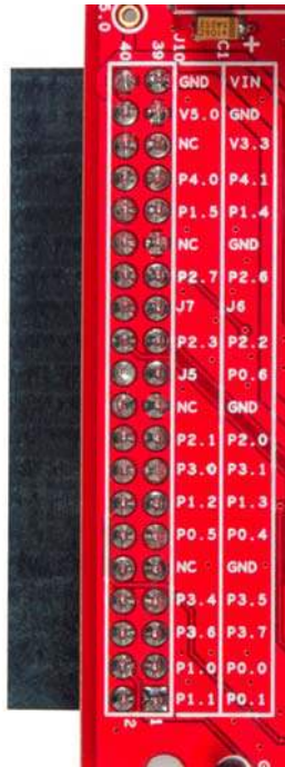
Figure 4-7. Pinout Selections of 40-Pin Header
