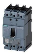
circuit breaker 3VA5 UL frame 125 breaking capacity class S 25kA @ 480 V 3-pole, line protection TM230, FTAM, In=15A overload protection Ir=15A fixed short-circuit protection Ii=10...20 x In UL489 SB (naval), 50 deg. cel. nut keeper kit on both sides
