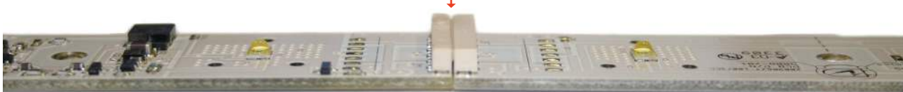
Figure 1 (6) CREE XP-G LEDs in series (V = 24VDC) and end-feeding another strip
