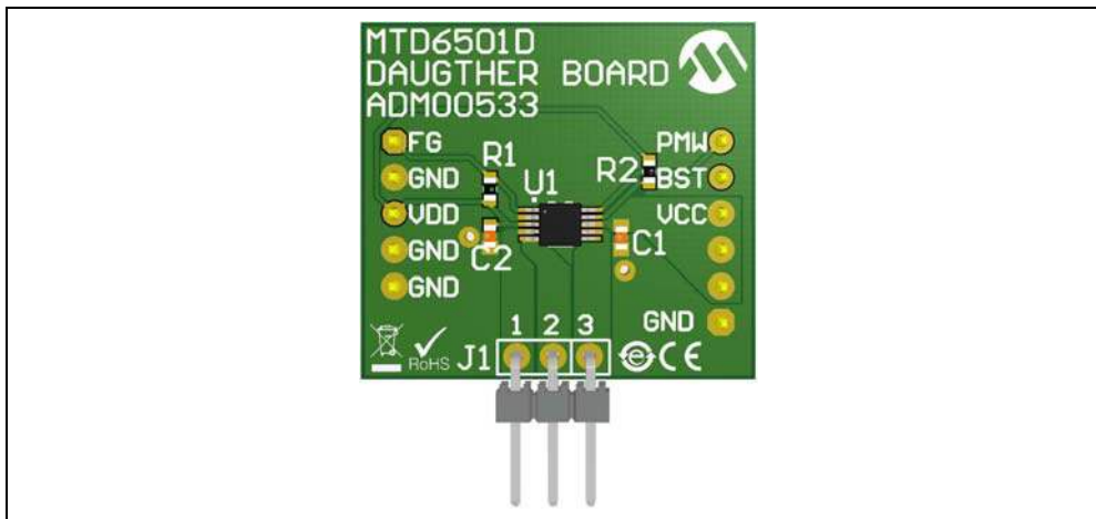
FIGURE 1-2: MTD6501D 12V 3-Phase BLDC Sensorless Fan Controller Daughter Board User's Guide Overview.
