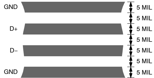
Figure 4. Typical Arrangement of Signal Tracks
